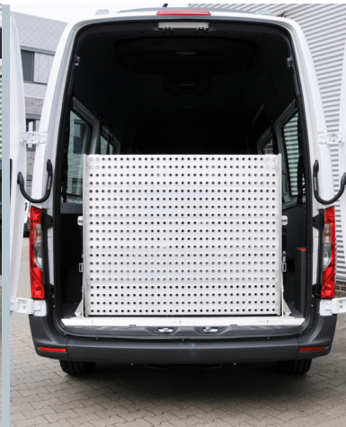
Vehicle with folded ramp. Rear view is maintained.
